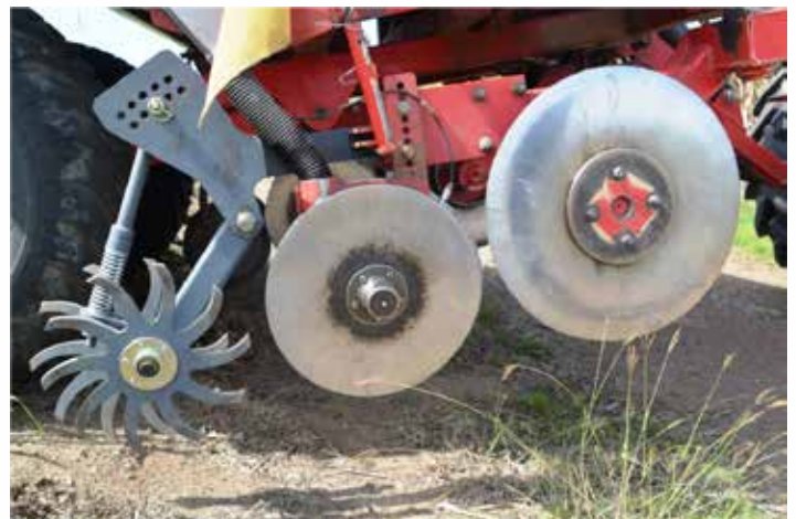
The StoolZippa helps ensure effective incorporation of nitrogen fertilisers to reduce volatilisation potential.
